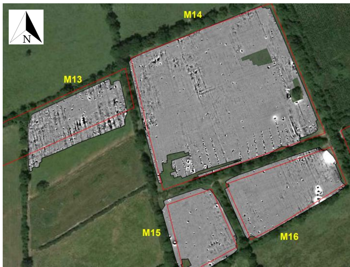
Figure 8: Greyscale imagery from the geophysical survey (24R0297) of the fields within the substation area (after Nicholls, 2024)
